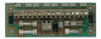
The **QE20-FP2027 Fused Power Distribution Board** provides 4 separately fused 24VDC outputs for wiring to other equipment inside the QE20 panel or to equipment outside the cabinet that must be powered by the QE20.
